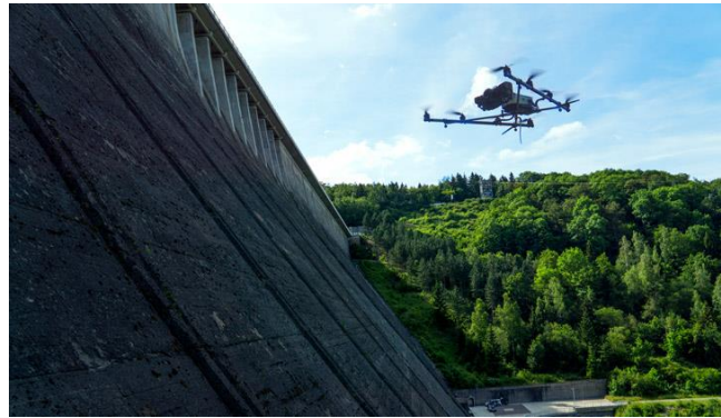
Fig.1 The use of a drone to inspect a dam [8]
